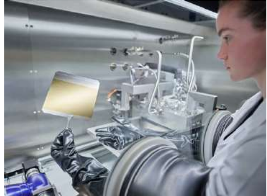
A spatial ALD tool equipped with glove box to deposit high quality SnO 2 films. Source: Peter Visser - SALD
