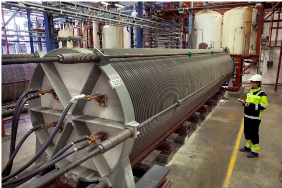
One of the four electrolyzers at the Nouryon plant in Rjukan, Norway
